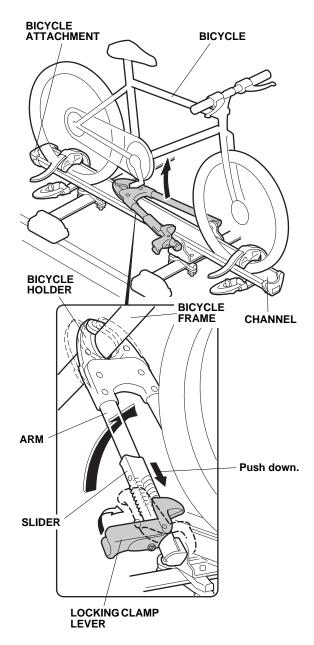
11. Push up the locking clamp lever to secure the bicycle frame.
